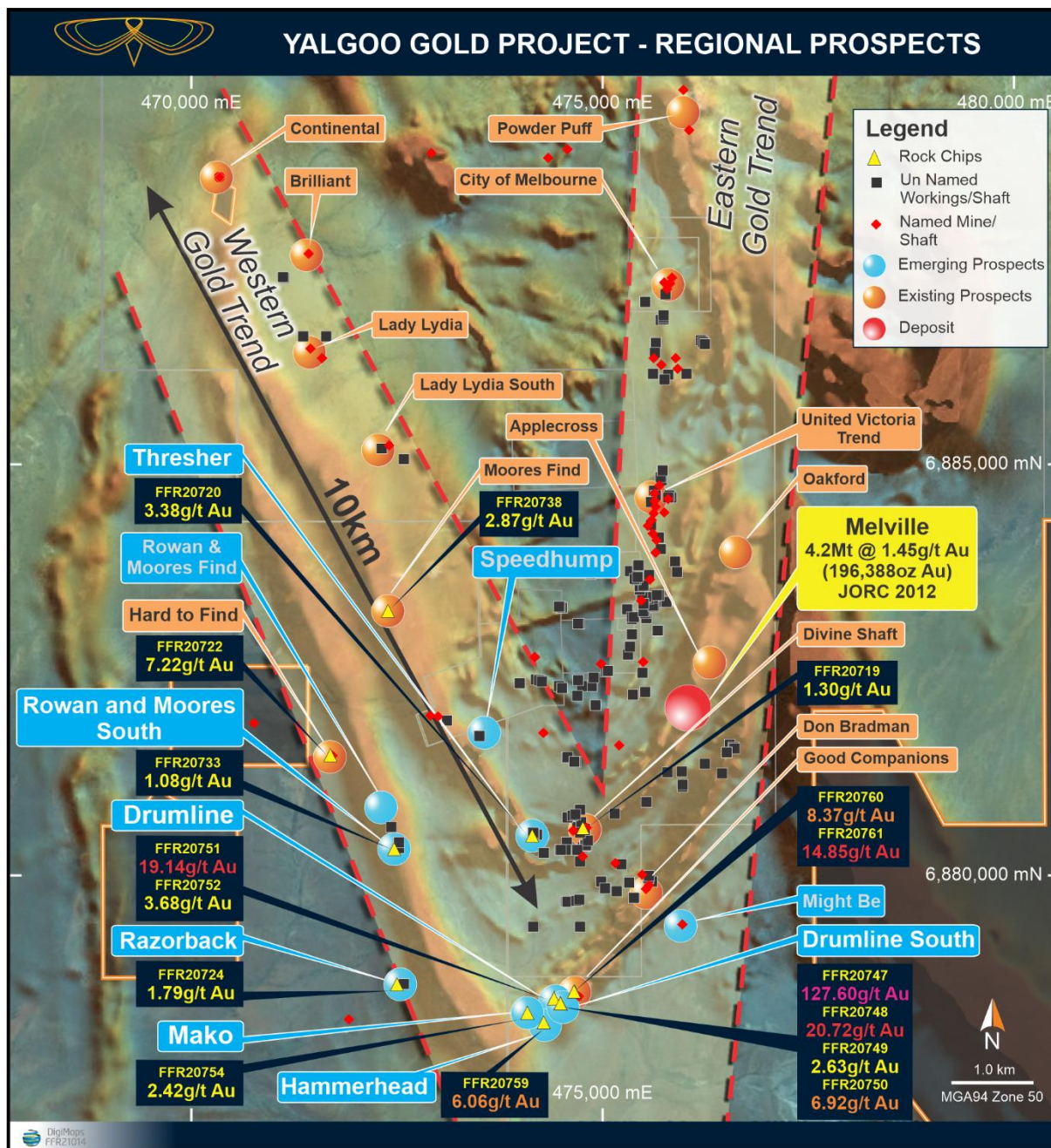
Figure 1. Plan view of northern Yalgoo Gold Project illustrating the widespread gold mineralisation that Firefly has defined as the Western and Eastern Gold Trends. Of particular note are the numerous workings at the intersection of the two gold trends and the very high-grade assays reported from this area in this announcement.
