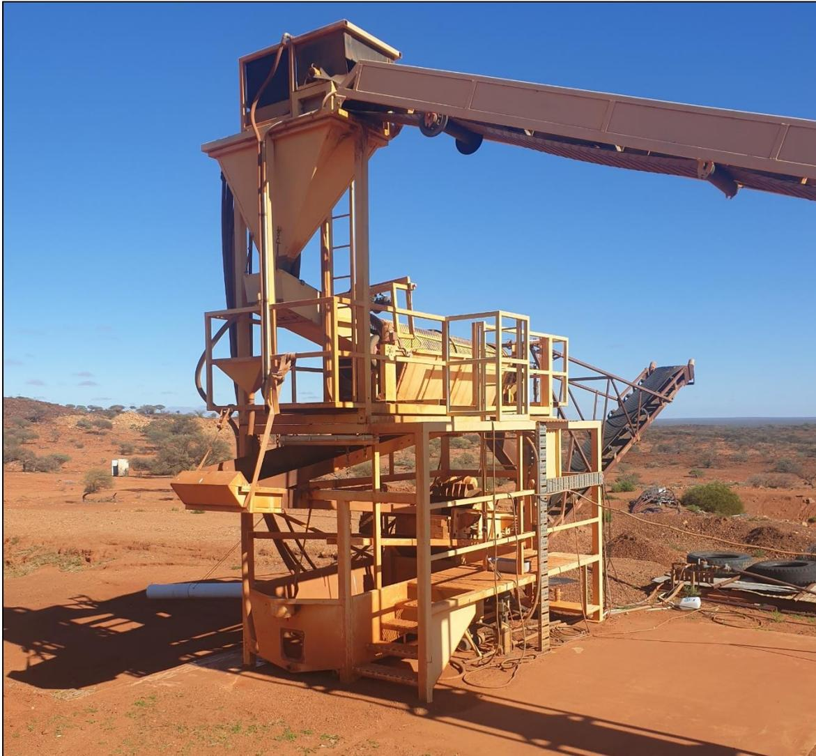
**Figure 3.** Fully operational 25-30tph “wash-plant” acquired as part of the acquisition.
