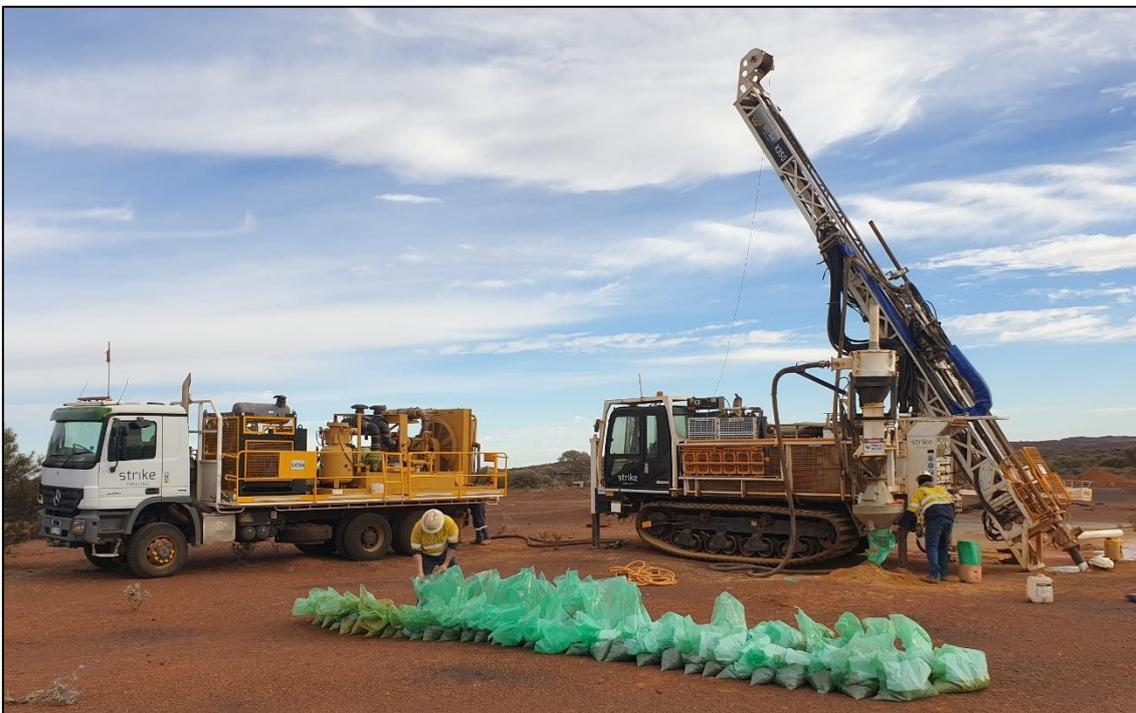
**Figure 1.** Strike Drilling Reverse Circulation track-mounted drill rig (Rig 04) operating at the Yalgoo Gold Project over the weekend.
